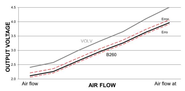
The red lines indicate the error in a DUT (Device Under
